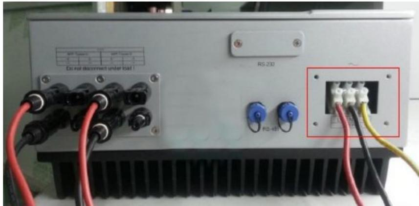
Fig.1 AC cables wiring
